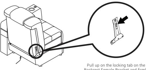
Pull up on the locking tab on the Backrest Female Bracket and firmly pull the backrest upward.
