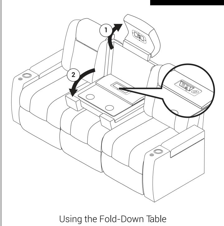
Lift the headrest then pull down on the backrest to open the Fold-Down Table. Push the button on the USB/110V Panel to access it. Push the USB/110V Panel shut when returning the Fold-Down Table to its upright position.
